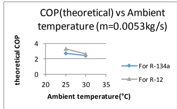
The above graph show that theoretical COP decreases with increase in the ambient temperature, whereas for same ambient temperature COP of R-12 is higher than R-134a
