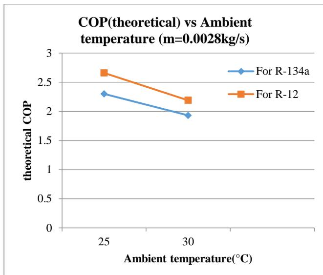
The above graph show that theoretical COP decreases with increase in the ambient temperature, whereas for same ambient temperature COP of R-12 is higher than R-134a.
