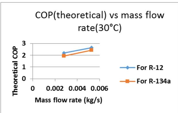
The above graph show that with increase in mass flow rate theoretical COP increases, whereas for the same mass flow rate COP of R-12 is higher than R-134a
