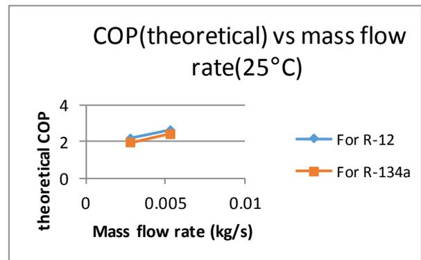
The above graph show that with increase in mass flow rate theoretical COP increases, whereas for the same mass flow rate COP of R-12 is higher than R-134a
